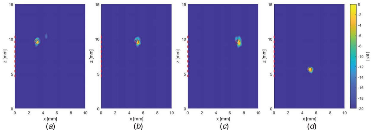
**Fig. 9** TFM images generated for clusters of defects located at  $+2\ \text{mm}$  from the center of the array and a depth of (a)  $3\ \text{mm}$ , (b)  $5\ \text{mm}$ , and (c)  $7\ \text{mm}$ . A cluster at  $-2\ \text{mm}$  and a depth of  $5\ \text{mm}$  is shown in (d). In all cases, the defect cluster location is highlighted with a circle, and the phased array location is highlighted with a dashed line.
