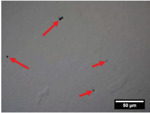
**Fig. 2** Representative image showing porosity within samples printed with the OEM recommended setting of 200 W laser power
