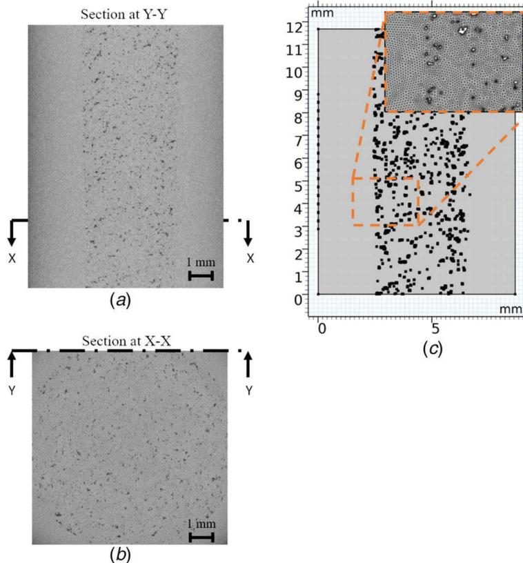
**Fig. 5** (a) Front and (b) top cross sections of an X-ray CT scan of Sample 2 showing a uniform distribution of the defects in the core region. (c) Defect geometry as generated from the XCT images to be used in FEM wave propagation simulations.
