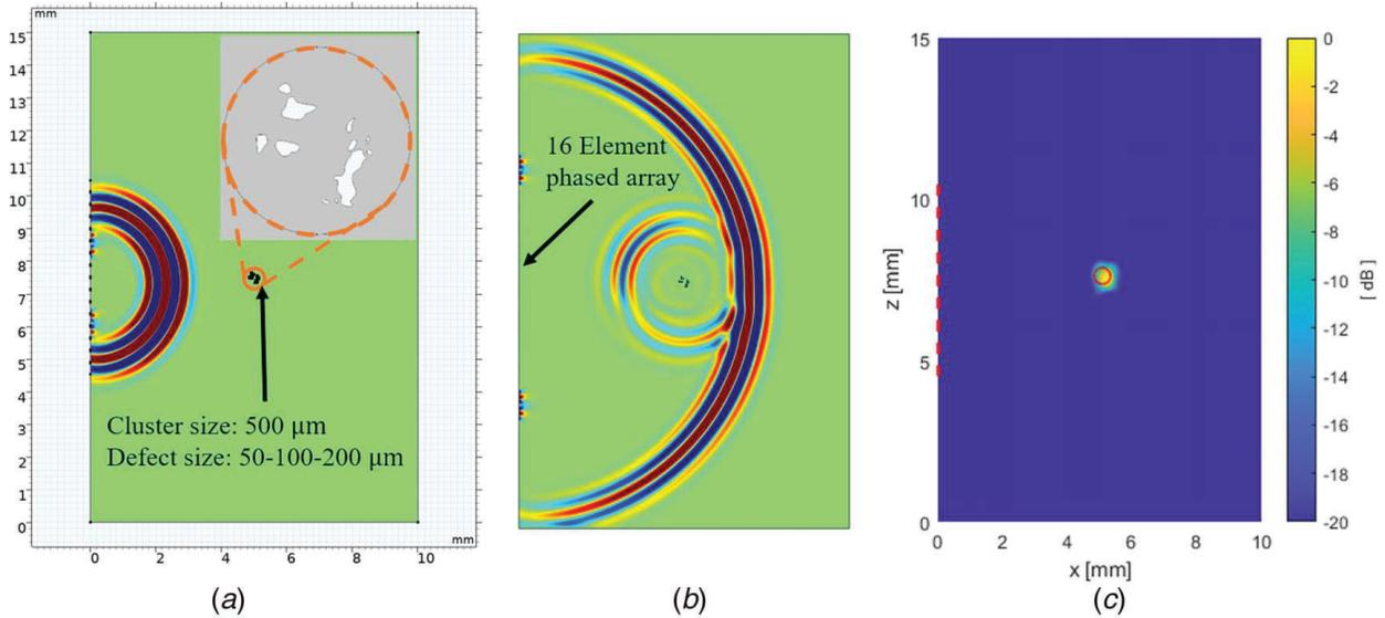
**Fig. 8** (a and b) Two time snapshots showing the propagation and reflection of longitudinal waves generated by a single phased array element and reflected from a cluster of defects of size  $500\ \mu\text{m}$  located at  $5\ \text{mm}$  depth. (c) The TFM image as constructed from the FMC data of the phased array shown in (b). The cluster of defects location is highlighted with a circle.
