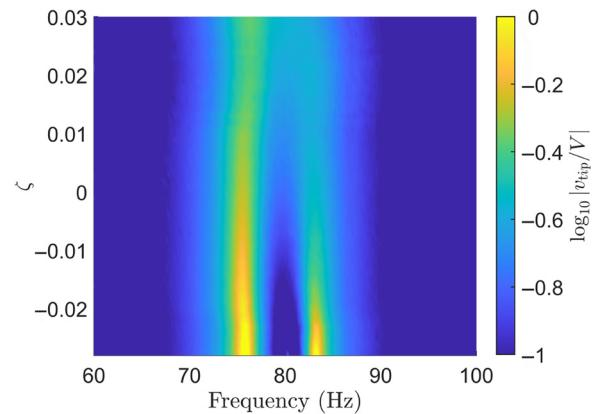
FIG. 2. The experimental tip-velocity FRF for a resonant shunt with  $f_t = 78 \text{ Hz}$  and varying damping ratio  $\zeta$ . Due to freedom of design with synthetic impedance, the damping ratio specified by the circuit can be made negative to cancel the inherent damping present in the structure and circuit. The system becomes unstable near  $\zeta = -0.028$ .
