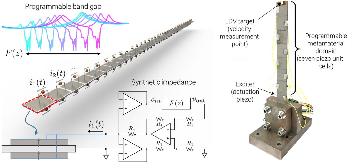
FIG. 1. Left: a schematic of the programmable piezoelectric locally resonant metamaterial with a digitally tunable band gap. Thickness-poled piezoelectric patches are connected in parallel for bending vibration and shunted to synthetic impedance circuits, which have an impedance determined by the digital transfer function  $F(z)$ . This enables the creation of a fully programmable locally resonant band gap. Right: the experimental realization of the programmable resonant metamaterial.
