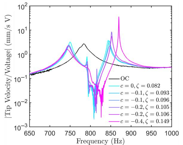
FIG. 4. The measured FRFs for  $\omega_t/(2\pi) = 780$  Hz with four different negative capacitance values and various damping ratios. Note that higher damping ratios are required to maintain stability at more negative values of  $c$ . The open circuit response is shown for reference.
