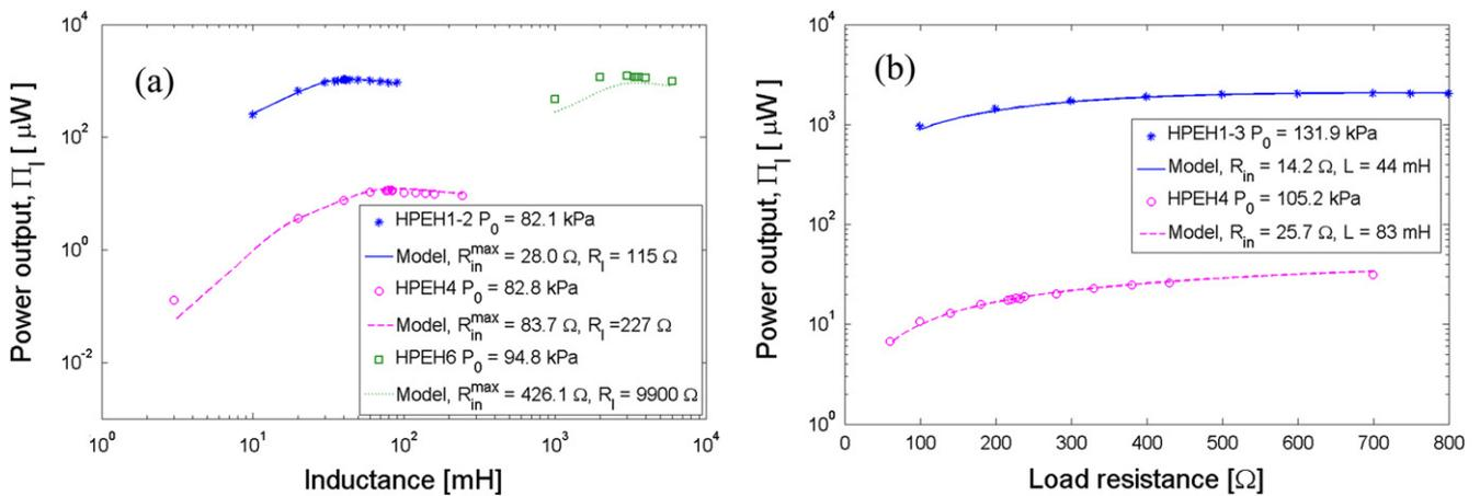
**Figure 7.** HPEH device power comparison for different devices versus load (a) inductance and (b) resistance.
