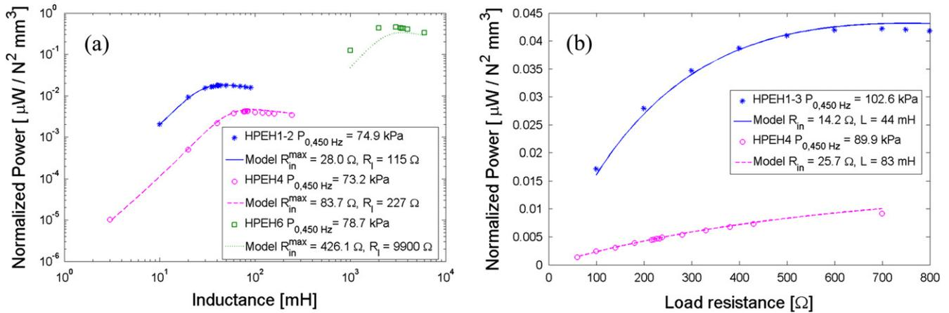
**Figure 6.** HPEH power delivered to the resistive load normalized by force and stack volume versus load (a) inductance and (b) resistance (ripple frequency: 450 Hz).
