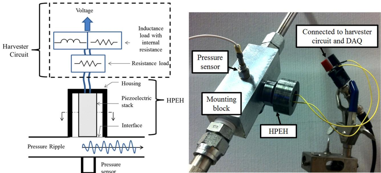
**Figure 1.** HPEH schematic including a resistive-inductive energy harvesting circuit and a picture of the experimental setup.
