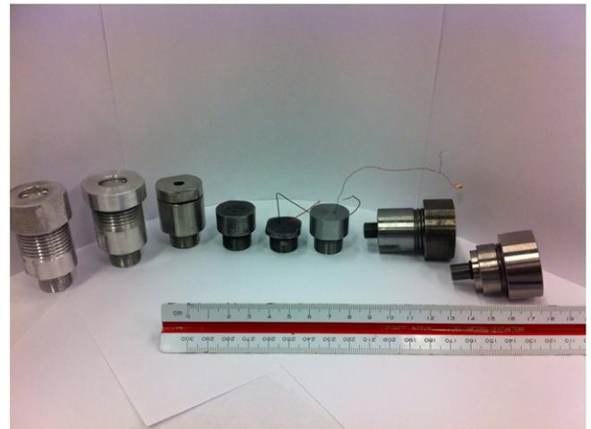
**Figure 5.** HPEH devices tested in this work (from left to right: 1-2, 2, 3-1, 3-2, 4, 6, 1-3, and 5).
