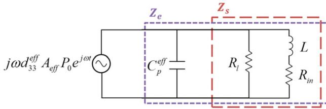
**Figure 2.** Circuit model for a HPEH device shunted to a resistive-inductive load with internal resistance of the inductor (current source in parallel with internal capacitance and shunt impedance).
