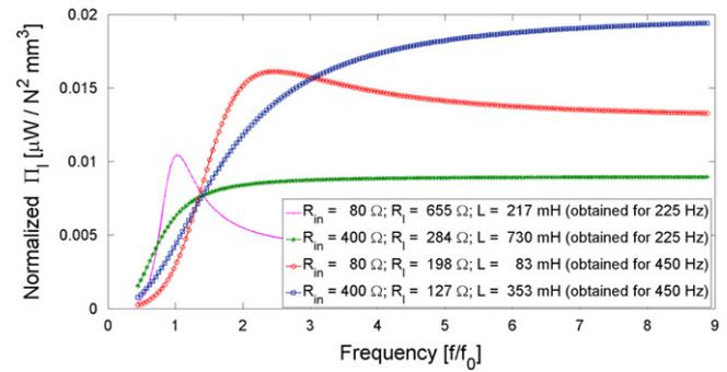
**Figure 4.** Normalized power versus frequency for different parameter combinations ( $d_{33}^{eff} = 182.9$  nC N $^{-1}$ ,  $C_p^{eff} = 3.08$   $\mu$ F,  $f_0 = \omega_0/2\pi = 225$  Hz).
