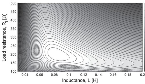
**Figure 3.** Normalized power density versus load resistance and inductance (for  $R_{in} = 80 \Omega$ ,  $f = \omega/2\pi = 450$  Hz,  $d_{33}^{eff} = 182.9$  nC N $^{-1}$ , and  $C_p^{eff} = 3.08$   $\mu$ F).
