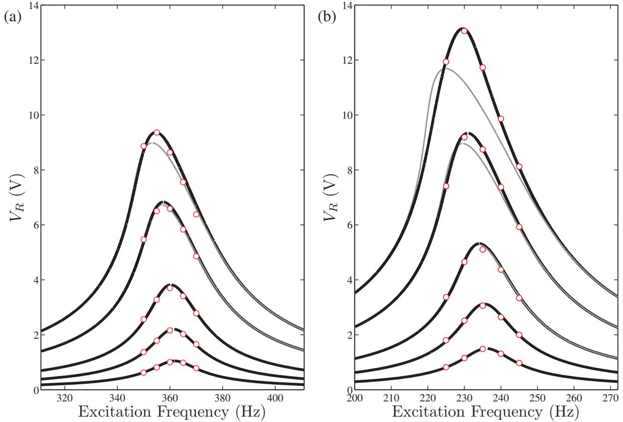
**Figure 6.** Experimental data points (circles), identified nonlinear resonance curves with fifth-order nonlinearities (black lines), and the cubic model predictions (gray lines) for the PZT-5H bimorph with (a)  $M_t = 0.24$  kg and (b)  $M_t = 0.787$  kg. The excitation levels shown are 0.145 g, 0.31 g, 0.56 g, 1.12 g, and 1.7 g.
