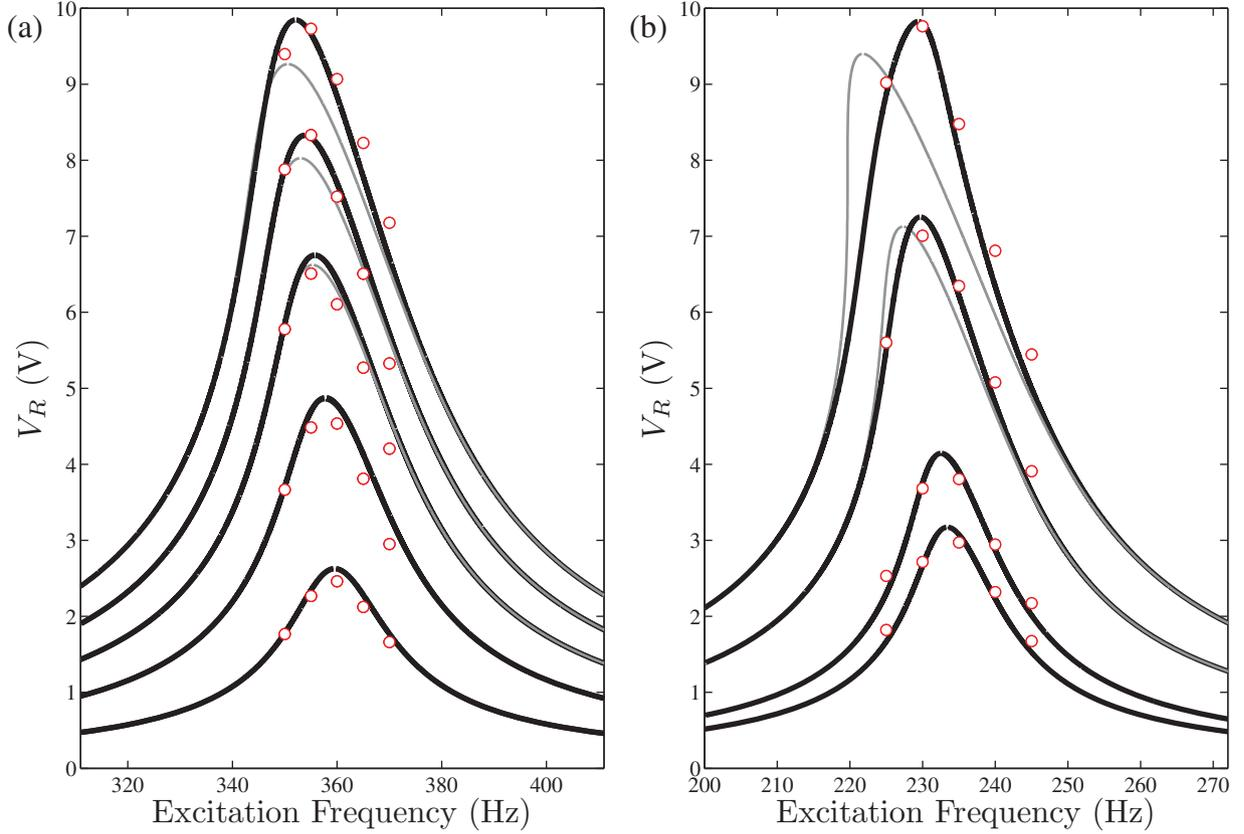
**Figure 7.** Experimental data points (circles), identified nonlinear resonance curves with fifth-order nonlinearities (black lines), and the cubic model predictions (gray lines) for the PZT-5A bimorph with (a)  $M_t = 0.24$  kg and (b)  $M_t = 0.795$  kg. The excitation levels in (a) are 0.4 g, 0.8 g, 1.2 g, 1.6 g, and 2 g, while in (b), we show 0.3 g, 0.4 g, 0.8 g, and 1.2 g.
