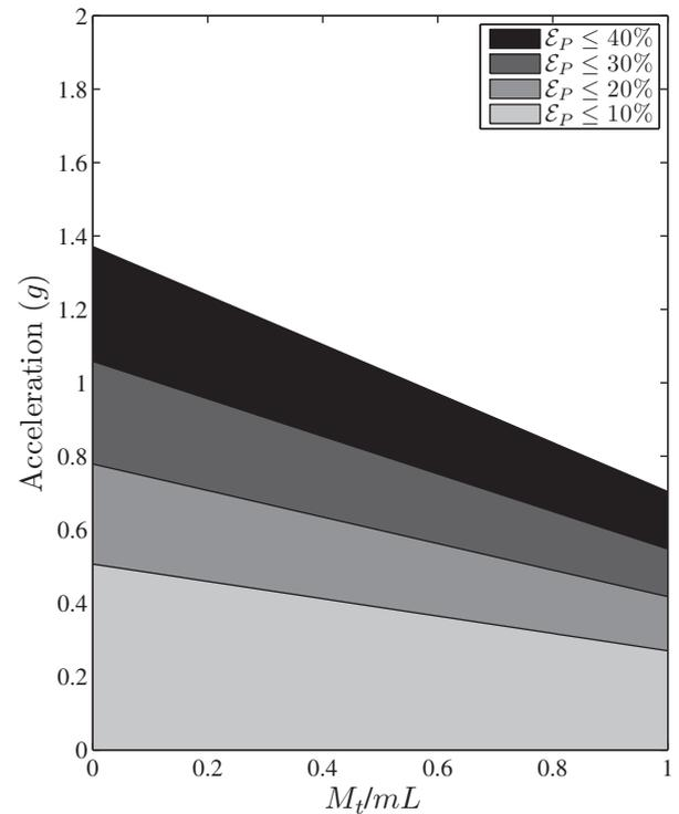
**Figure 12.** Influence of the mass ratio  $\alpha$  and base acceleration on the linear model error for the predicted power of the PZT-5A bimorph.
