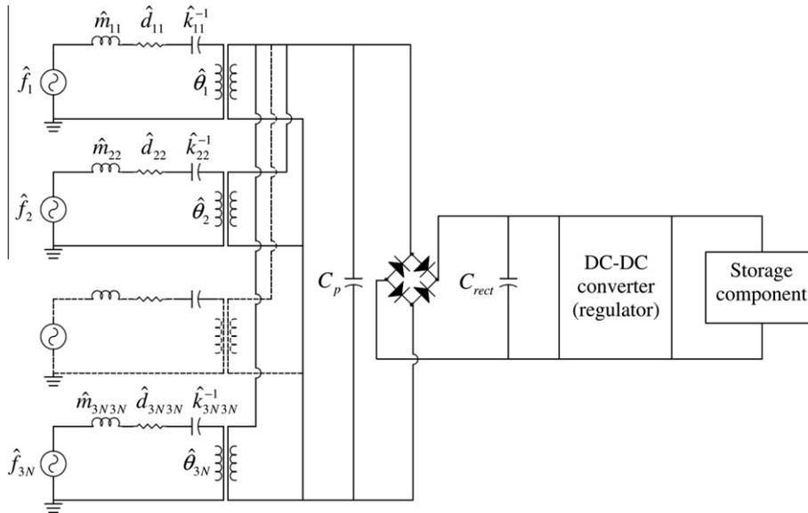
**Fig. 12.** Schematic of a unimorph piezoelectric energy harvesting and storage system based on the Timoshenko model of the cantilever as components on the left-hand-side of the transformers for each assumed mode in decoupled generalized coordinates, an AC–DC converter (full-wave rectifier with a smoothing capacitor), a DC–DC converter, and a storage component.
