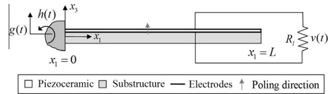
Fig. 1. Unimorph piezoelectric energy harvester with varying cross-section.
