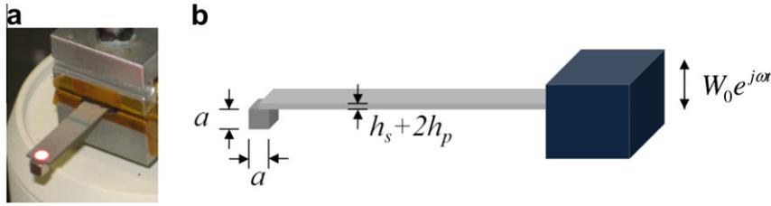
Fig. 9. Bimorph cantilever after the addition of the cube-shaped tip mass: (a) close-up view and (b) schematic.
