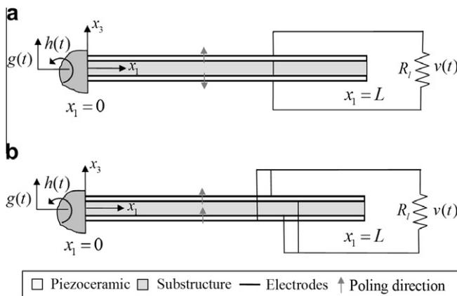
**Fig. 2.** Bimorph piezoelectric energy harvester configurations with symmetric laminates and varying cross-section: (a) series connection and (b) parallel connection.
