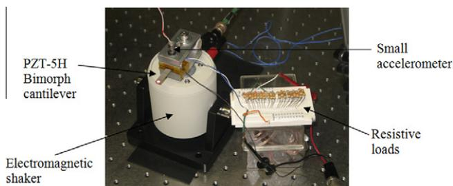
Fig. 3. Experimental setup showing the brass-reinforced PZT-5H bimorph cantilever clamped to the armature of a shaker and a set of resistive loads.
