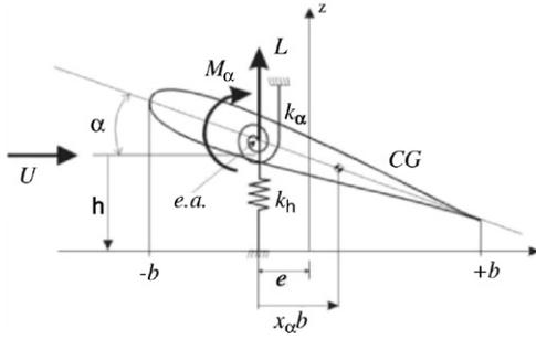
**Figure 1.** 2-DOF typical aeroelastic section under airflow excitation.
