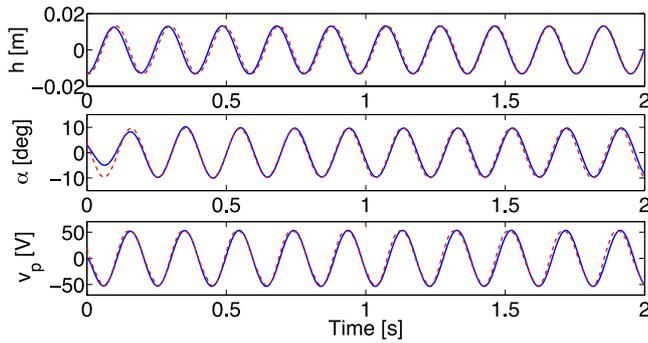
**Figure 7.** Experimental (dashed line) and theoretical (solid line) nonlinear piezoaeroelastic response histories for  $R_1 = 100 \text{ k}\Omega$  (experiment:  $10.0 \text{ m s}^{-1}$ , model:  $10.4 \text{ m s}^{-1}$ ).
