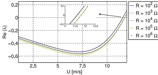
**Figure 4.** Real part of the eigenvalue (for the mode that becomes unstable) with increasing airflow speed for a set of resistive loads along with a close-up view around the flutter boundary.
