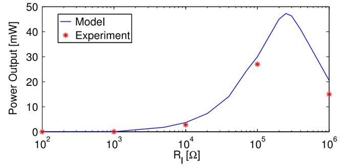
**Figure 8.** Experimental and theoretical power outputs versus load resistance (experiment:  $10.0 \text{ m s}^{-1}$ , model:  $10.4 \text{ m s}^{-1}$ ).
