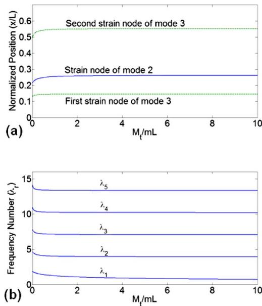
**Fig. 4** (a) Variation of the strain node positions of the second and the third vibration modes and (b) variation of the first five frequency numbers with tip mass-to-beam mass ratio
