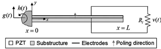
**Fig. 1 Piezoelectric energy harvester under translational and small rotational base excitations**
