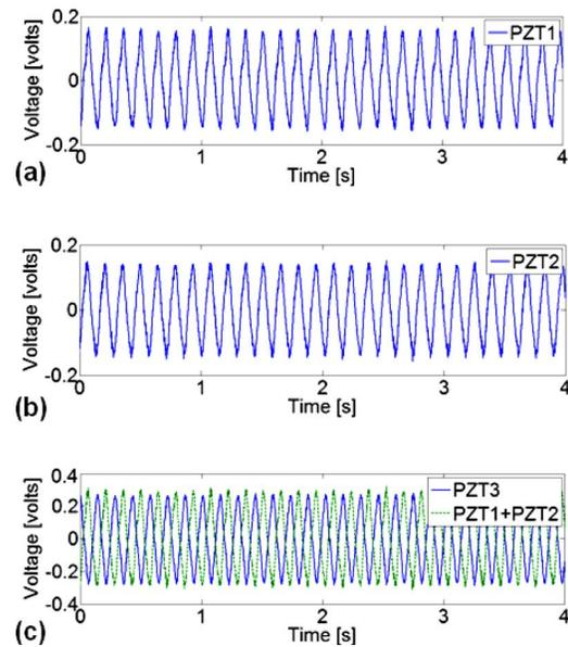
**Fig. 6 Voltage histories for excitation at the first natural frequency of the beam: (a) PZT1, (b) PZT2, and (c) PZT3 along with the maximum response obtained by combining PZT1 and PZT2**
