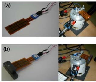
**Fig. 9** Piezoelectric bimorph and its experimental base excitation with a shaker in clamped-free boundary conditions: (a) without a tip mass and (b) with a tip mass
