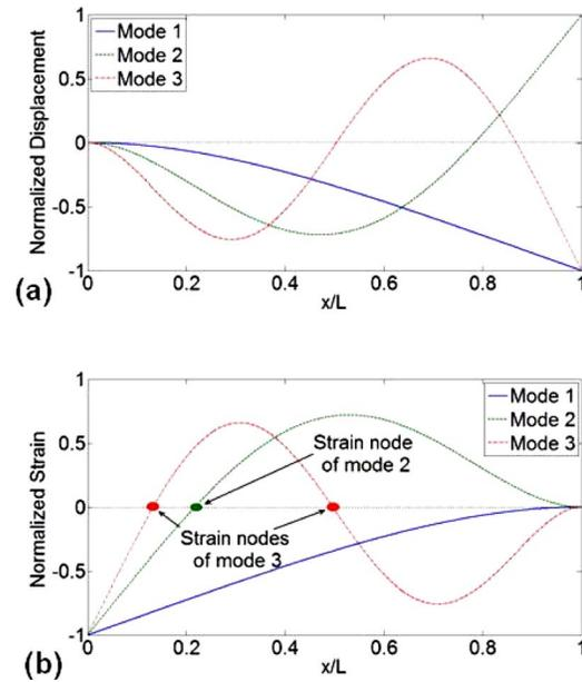
**Fig. 2 (a) Normalized displacement and (b) normalized strain mode shapes of a cantilevered beam without a tip mass for the first three vibration modes**
