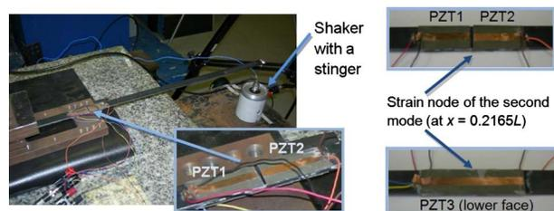
**Fig. 5 Experimental setup for demonstration of the effect of strain nodes on the voltage output**
