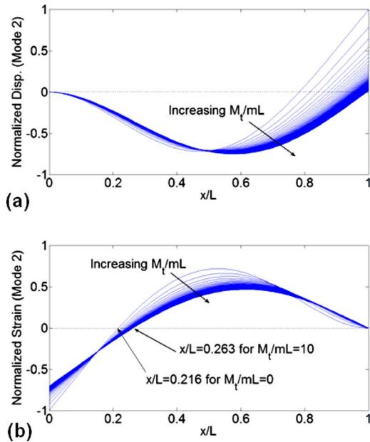
**Fig. 3** Variation of the (a) normalized displacement and (b) normalized strain mode shapes of the second vibration mode with tip mass-to-beam mass ratio
