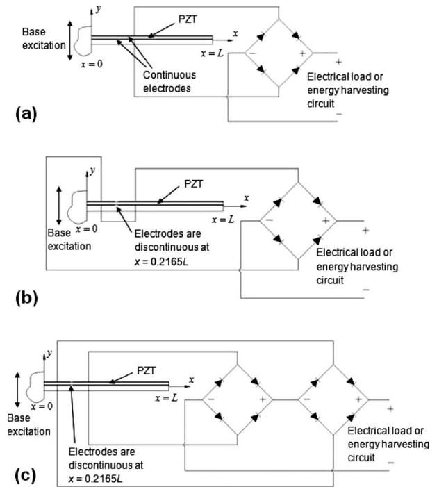
**Fig. 8 Continuous and segmented electrode configurations with full-wave rectifiers: (a) suitable for mode 1 excitation, (b) suitable for mode 2 excitation, and (c) suitable for both mode 1 and mode 2 excitations**
