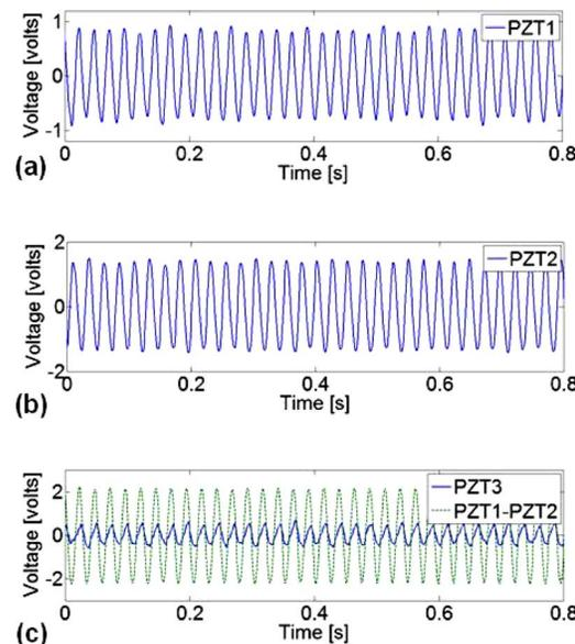
**Fig. 7 Voltage histories for excitation at the second natural frequency of the beam: (a) PZT1, (b) PZT2, and (c) PZT3 along with the maximum response obtained by combining PZT1 and PZT2**
