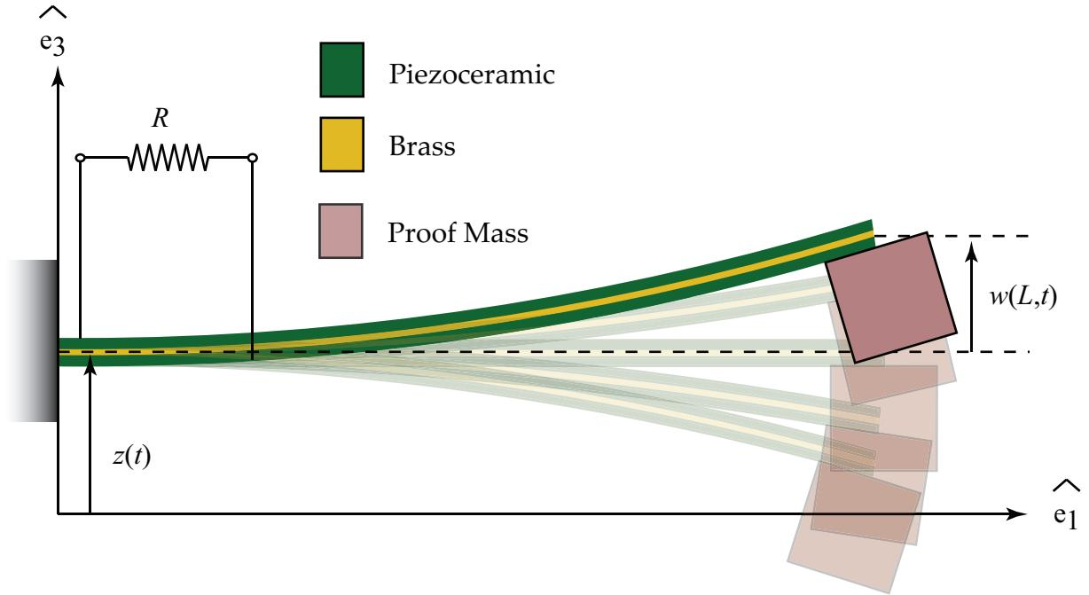
**Figure 1.** Illustration of the energy harvester studied. The cantilever is excited by a base motion  $z(t)$  and transversely deflects a distance of  $w(x, t)$ .
