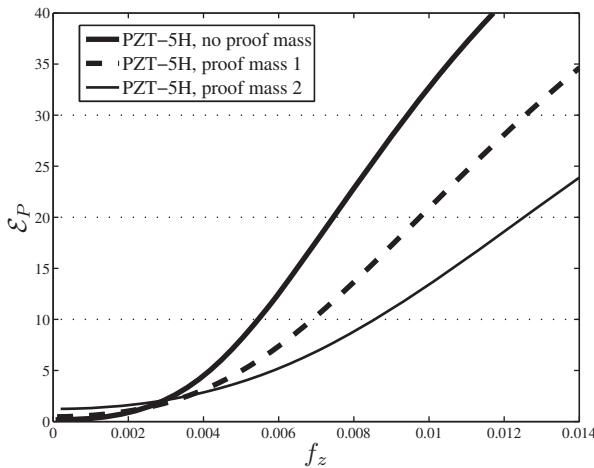
**Figure 9.** Error in predicted power due to linear piezoelectricity assumptions for the PZT-5H bimorph.
