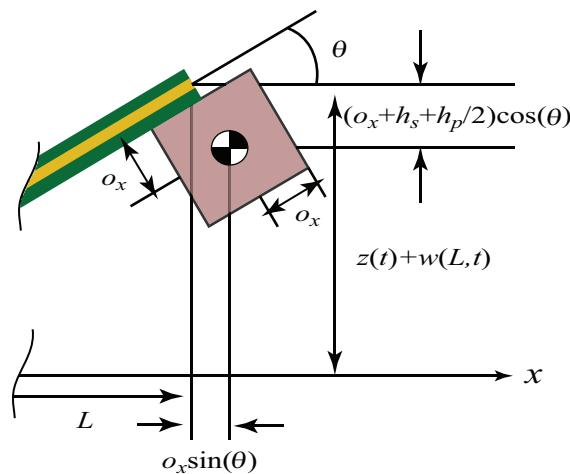
**Figure 2.** Closer view of the proof mass kinematics for determining the position vector from the origin to the center of mass.
