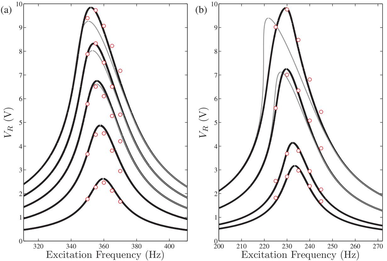
**Figure 7.** Experimental data points (circles), identified nonlinear resonance curves with fifth-order nonlinearities (black lines), and cubic model predictions (gray lines) for the PZT-5A bimorph with (a)  $M_t = 0.24$  kg and (b)  $M_t = 0.795$  kg. The excitation levels in (a) are 0.4 g, 0.8 g, 1.2 g, 1.6 g, and 2 g, while in (b), we show 0.3 g, 0.4 g, 0.8 g, and 1.2 g.
