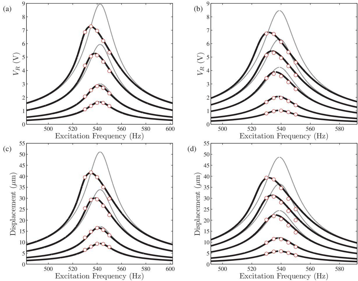
**Figure 5.** Experimental data points (circles), identified nonlinear resonance curves (black lines), and the linear model predictions (gray lines) for (a and c) PZT-5H and (b and d) PZT-5A bimorph with no attached proof mass. The excitation levels shown for PZT-5H are 0.3 g, 0.56 g, 1.12 g, and 1.6 g, and for PZT-5A, the excitation levels are 0.2 g, 0.4 g, 0.8 g, 1.2 g, and 1.6 g.
