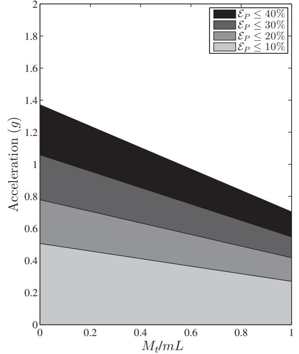
**Figure 12.** Influence of the mass ratio  $\alpha$  and base acceleration on the linear model error for the predicted power of the PZT-5A bimorph.
