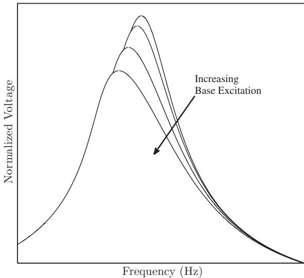
**Figure 3.** Illustration of the empirical trend in nonlinear resonance curves for the piezoelectric harvester. The output voltage is normalized by the drive amplitude to better portray the non-linear response.
