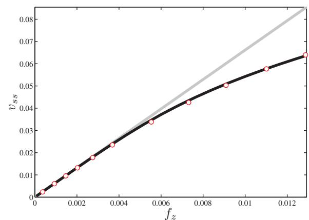
**Figure 8.** Experimental data points (red circles), nonlinear prediction (black line), and linear theory (gray line) for the voltage response at  $\Omega = 540$  Hz for the PZT-5H bimorph with no proof mass.
