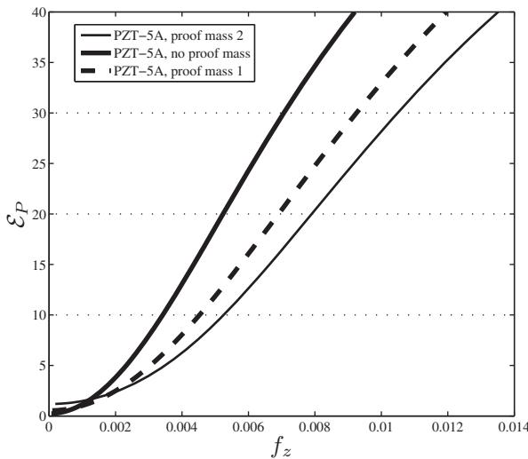
**Figure 10.** Error in predicted power due to linear piezoelectricity assumptions for the PZT-5A bimorph.
