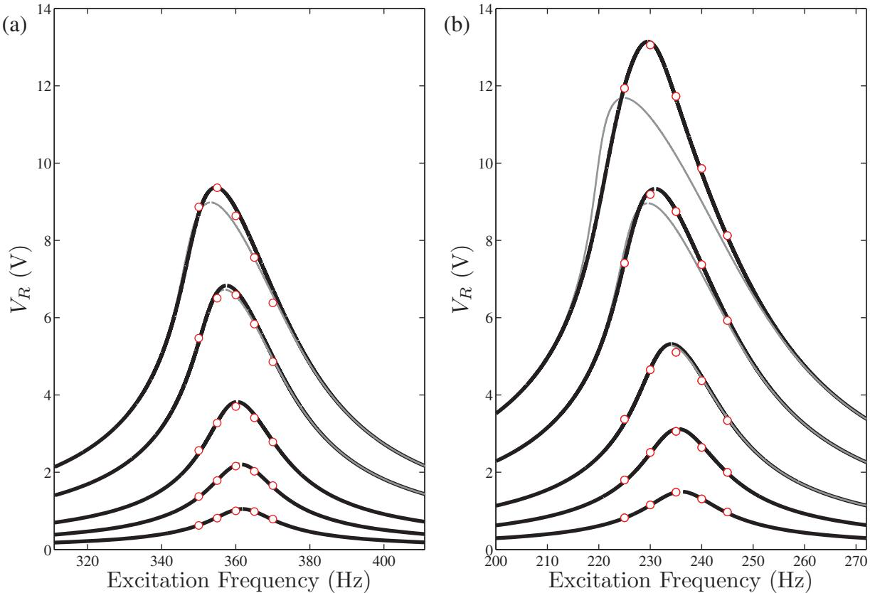
**Figure 6.** Experimental data points (circles), identified nonlinear resonance curves with fifth-order nonlinearities (black lines), and the cubic model predictions (gray lines) for the PZT-5H bimorph with (a)  $M_t = 0.24 \text{ kg}$  and (b)  $M_t = 0.787 \text{ kg}$ . The excitation levels shown are 0.145 g, 0.31 g, 0.56 g, 1.12 g, and 1.7 g.
