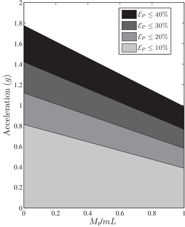
**Figure 11.** Influence of the mass ratio  $\alpha$  and base acceleration on the linear model error for the predicted power of the PZT-5H bimorph.
