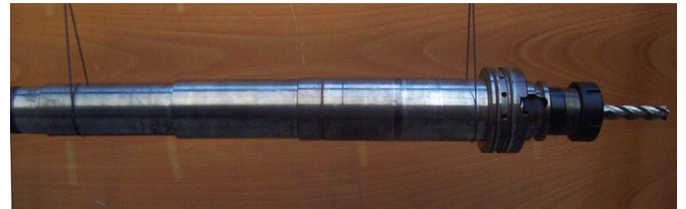
Fig. 6. Spindle–holder–tool suspended assembly for free–free measurements.
