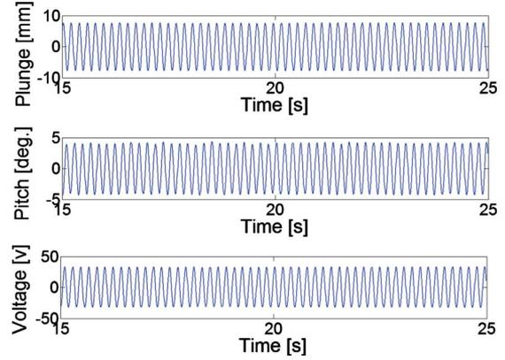
FIG. 3. (Color online) Experimental piezoaeroelastic response for  $R_l = 100$  k $\Omega$  and  $U_c = 9.30$  m/s.
