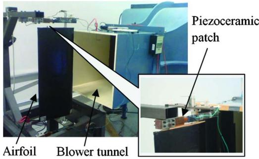
FIG. 2. (Color online) Experimental setup showing a typical aeroelastic section with piezoceramics attached onto the plunge stiffness members.
